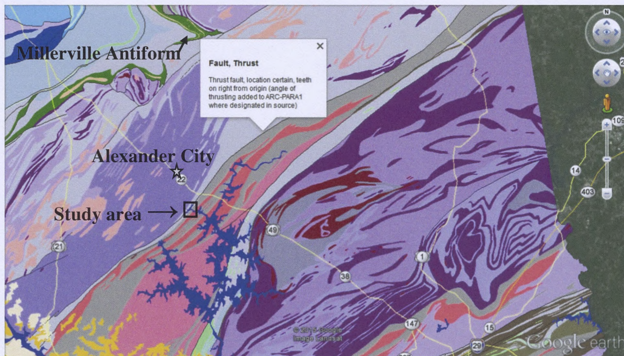
Figure 1. State geologic map of Alabama showing interpretation of the Alexander City fault as an extensive thrust fault at the structural top of the Elkahatchee Quartz Diorite along its contact with the overlying Wedowee Group, before cutting up section to become the boundary between the Wedowee Group and overlying Emuckfaw Group northeast of the Elkahatchee batholith. Adapted from Szabo et al. 1988.
