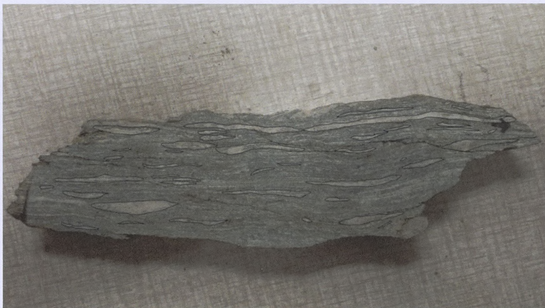
Figure 7. Rock samples were cut parallel to the mean stretching lineation and perpendicular to foliation, then photographed. Identifiable feldspar grains on each photograph were outlined by free-hand tracing their boundaries in PowerPoint.
